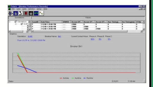
Trend graph and data table of the arcing and tripping time give you a clear picture what condition the breakers are.
